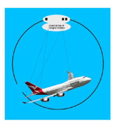
The box with the magnerall track would have to have a rigid cover like a thin perspex or board that cold be accurely attached to the box so that the magnets do not distort the surface as they are dragged around.
