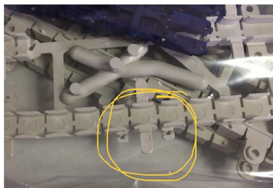
Arduino boards. By placing your track magnets east/west instead of the standard upright N/S position, the magnetic impulse will trigger the reed switch as that particular chain link passes by. Think of the multitude of things that could be activated - gates opened, traffic lights changed, stationary police car with their lights flash on as your vehicles approach, speed cameras flashing, people waving - the list goes on, with any animated scenery items triggered by the reed switch.
