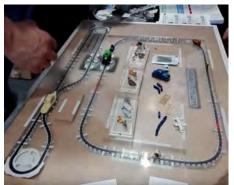
The Magnorail System operates on a simple plastic interlocking chain links travelling inside a flexible plastic channeling. Each link contains a cavity to take either a strong 3mm square rare earth magnet or a smaller cylindrical one for smaller scales, which then draws bicycles and vehicles along the track surface through normal magnetic properties. The central clear wheel with the cyclists feet attached creates the pedaling action through the articulated knee and hip joints.
